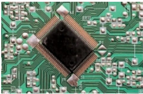
SN100C波峰焊接 Wave soldering with SN100C QFP100 pins 0.65mm pitch
