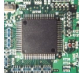
100 Pin(0.5mm pitch)QFP reflow soldered with SN96CI
